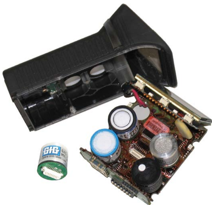
Figure 2: Multi-sensor instruments are able to use a wide range of sensors and detection technologies including O 2 , standard pellistor LEL, NDIR combustible gas and CO 2 , PID and over 20 different substance-specific electrochemical sensors for toxic gas measurement.
