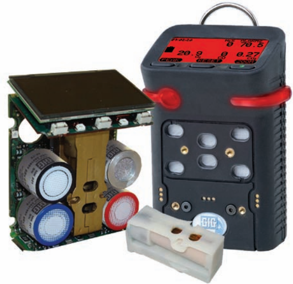
Figure 6: Instrument with NDIR sensor. Since the amount of IR light absorbed is proportional to the amount of target gas present, the longer the optical path-length through the IR sensor, the better the resolution.
