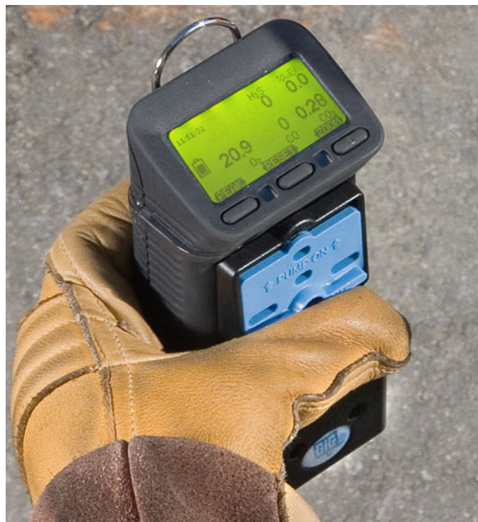
Figure 2: The only way to know whether an instrument is capable of proper performance is to expose it to test gas.
