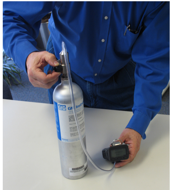
Figure 1: Performing a functional "bump test" by exposing the instrument to known concentration test gas takes only a few moments perform.
