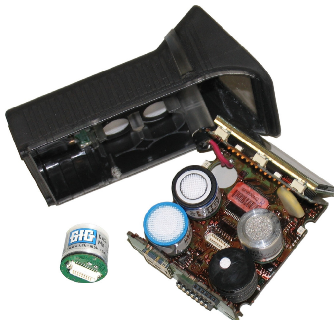
Figure 2: The G460 is able to use wide range of sensors and detection technologies including O 2 , standard pellistor LEL, NDIR combustible gas and CO 2 , PID and over 20 different substance-specific electrochemical sensors for toxic gas measurement.
