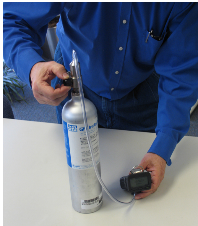
Figure 1: Performing a functional "bump test" by exposing the instrument to known concentration test gas takes only a few moments perform.
